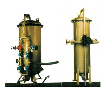
The raw water passes through a bed filled with small polystyrene beads known as ion exchange resins where sodium ions are exchanged for harness forming ions Once the beads are saturated with calcium and magnesium, the unit enters a regenerating cycle.
